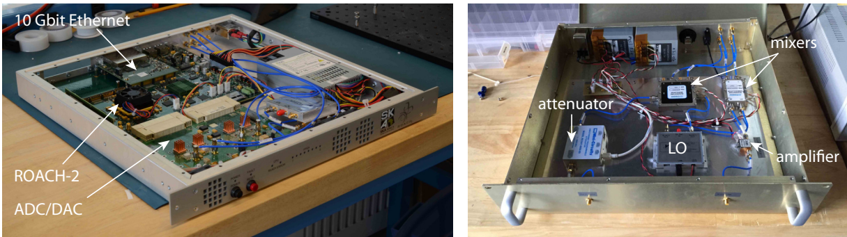
Figure C.3: (Left) A photograph of the ROACH-2 board. (Right) A photograph of the analog electronics box for the heterodyne readout system, including the local oscillator (LO). This figure was published in Johnson et al. [3].
